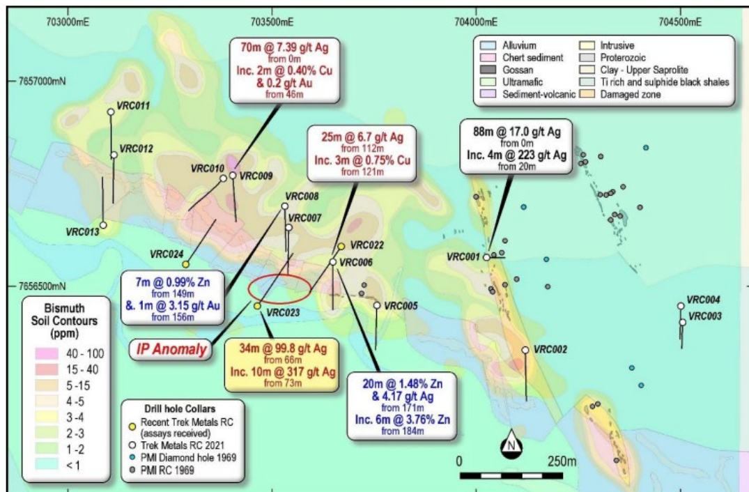
Figure 11 Valley of Gossans RC collars and intercepts
