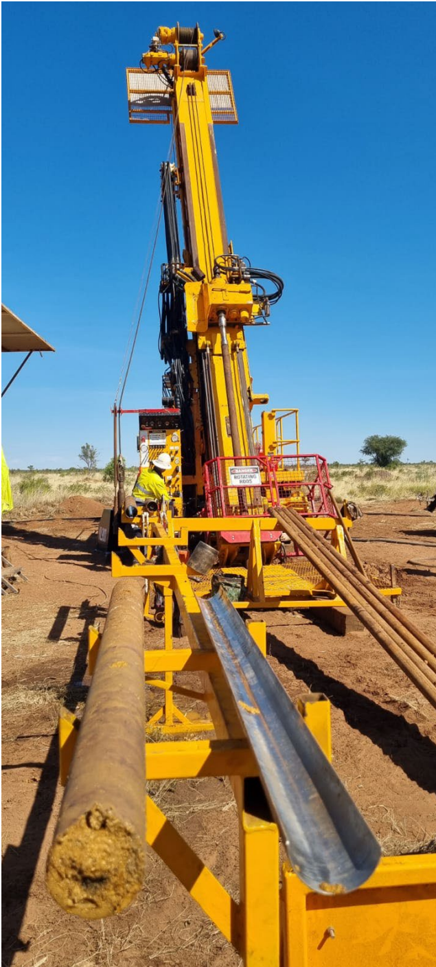
Figure 1: Kal Drill diamond rig with phosphate-rich PQ drill core
