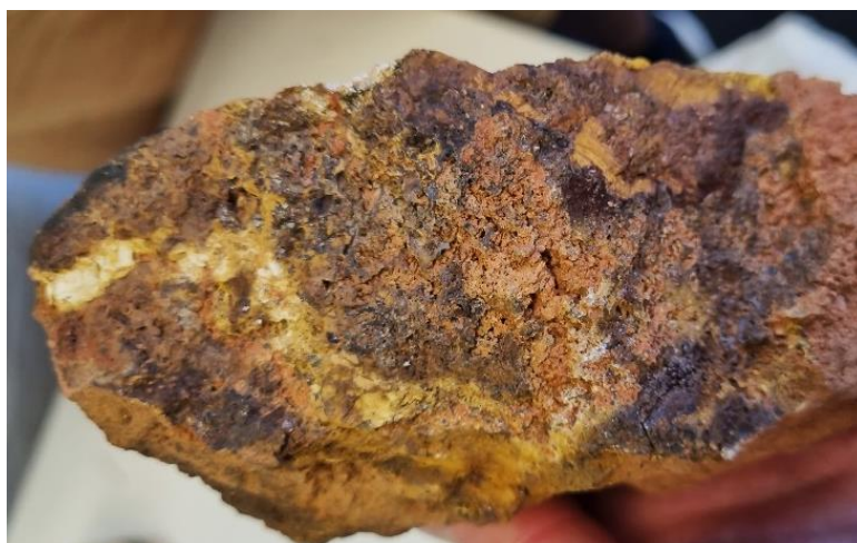
Figure 2 – (left) Field photograph of weathered carbonatite rock chip sample BY23K0360 assaying 1.1 % TREYO (22% NdPr), (right) Field photograph of weathered iron oxide rich pyroxenite or possible ferrocarbonatite rock chip sample LRBY21 with assays returning 263 ppm Sc203 and 0.7% TREYO (30% NdPr).
