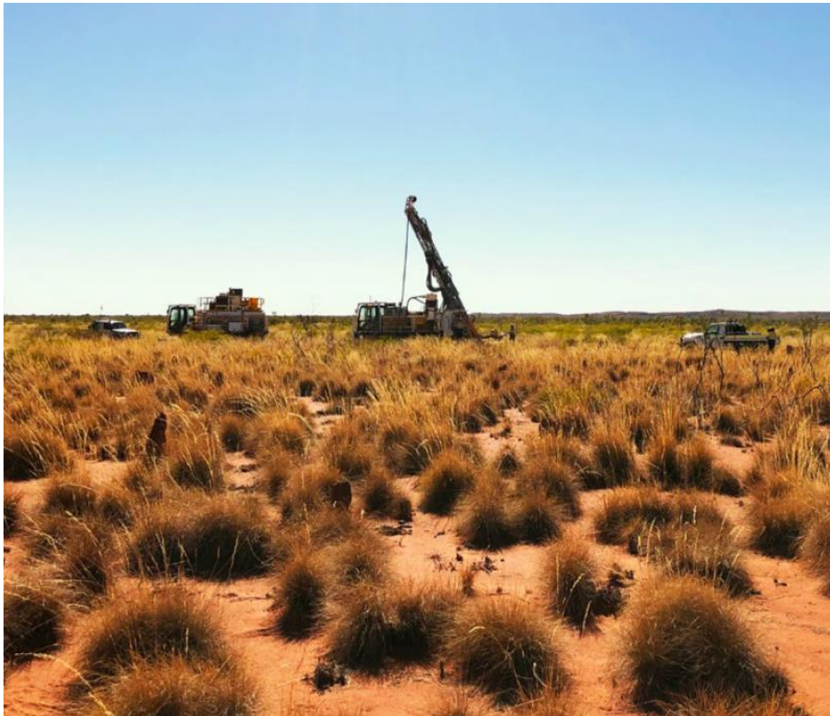
Figure 6. Drilling at Christmas Creek shows the dominant landscape of shallow transported cover. The next round of significant mineral discoveries is likely to come from under cover, such as at the Christmas Creek Project area. The work by Newmont has discovered multiple mineralised bedrock occurrences under the transported material.
