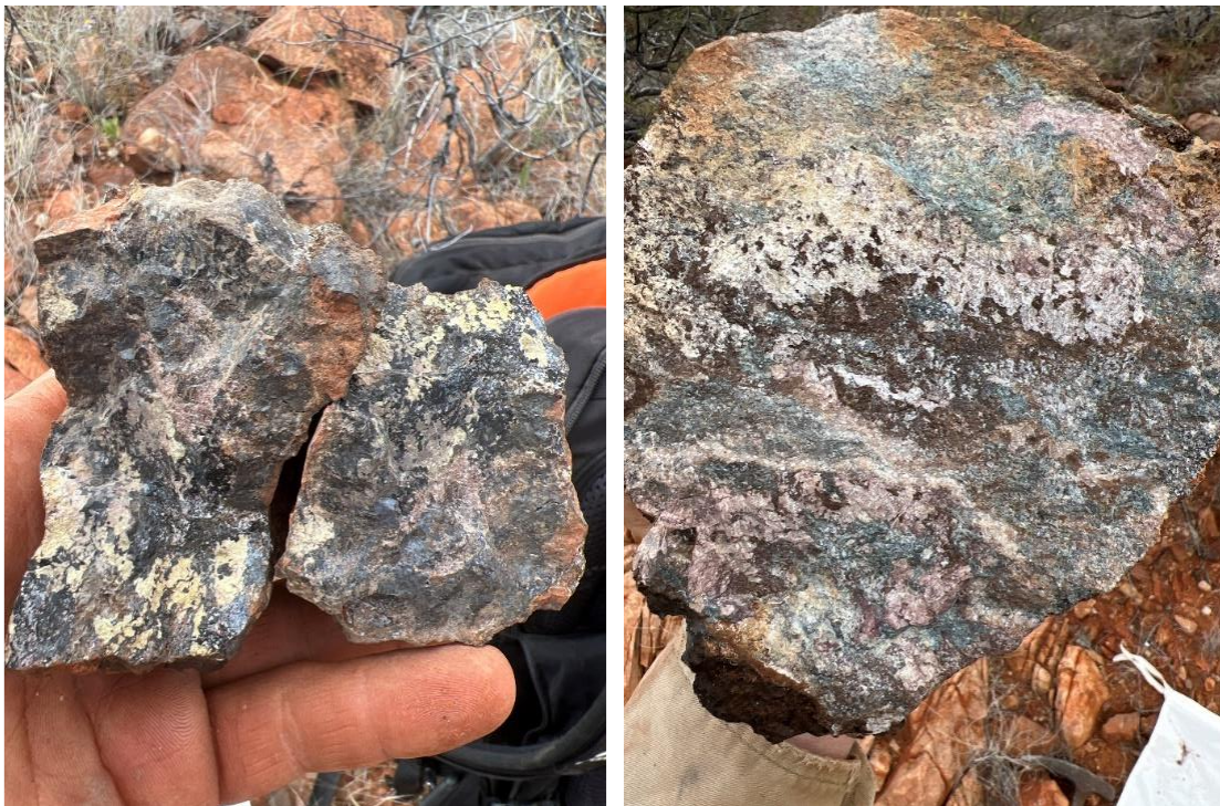
Figure 2: Monazite (pale red) rich carbonatite samples MWGS0769 (left) and MWGS0770 (right) which assayed 21.55% TREO with 3.74% Nd 2 O 3 + Pr 6 O 11 and 15.19% TREO with 2.56% Nd 2 O 3 + Pr 6 O 11 (see ASX:KFM 30 August 2022).
