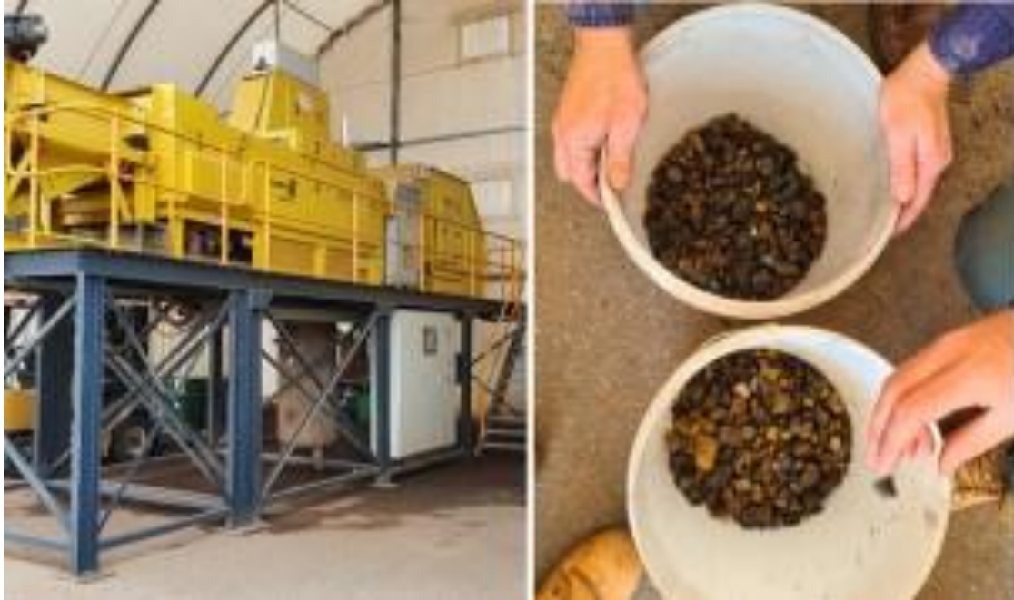
Figure 6. The Steinert ore sorter at Bibra Lake, Perth that was used to test +10mm samples from Hendeka (LHS) and the resultant material with Product top and Waste below (RHS).
