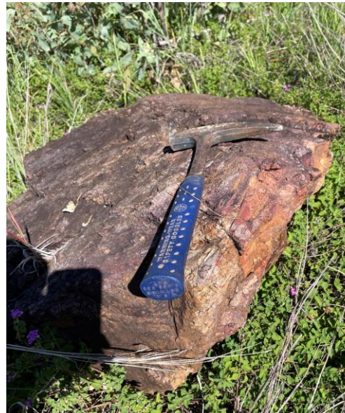
Sample BM2600 – rhyodacite breccia 0.05 g/t Au, 6.8 g/t Ag, 234 ppm As, 15.8 ppm Mo, 76.9 ppm Sb and 2.7 ppm Te
