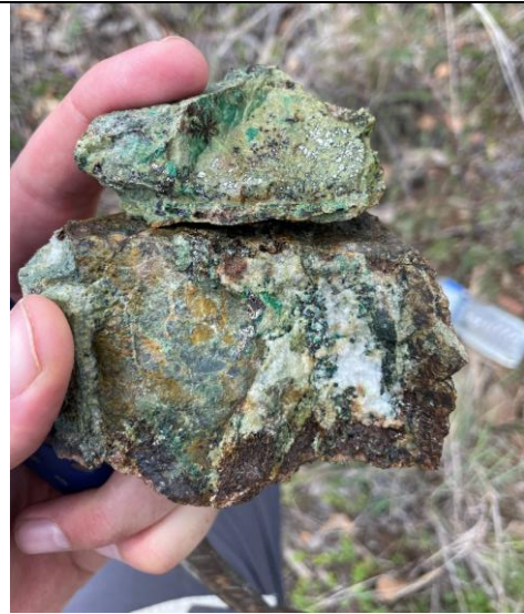
Sample BM2607 - quartz-sericite epidote alteration and malachite. Assayed 11.4 g/t Au and 1.2% Cu
