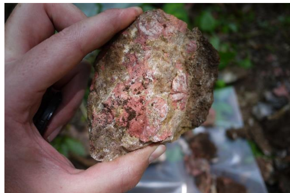
Figure 2. Sample 01 (K042532) for SEM and XRD results taken from Blue Jay prospect from sample above: assay results 3.6% TREO and 0.5% Nb 2 O 5 . Hosted in sovite.
