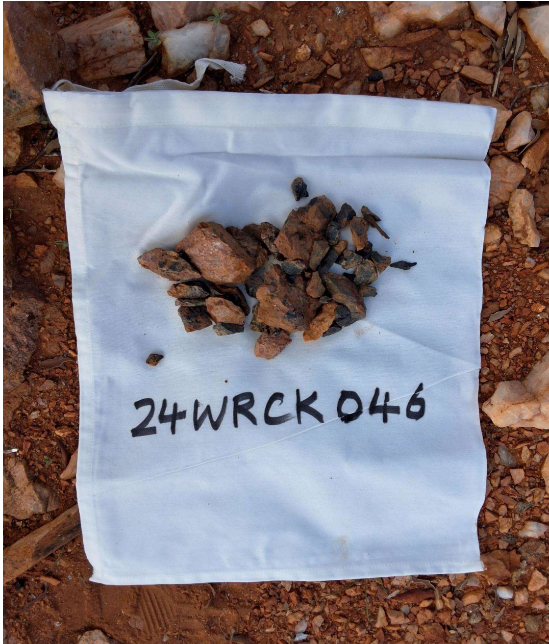
Figure 1: Large black rock fragments chipped directly from the in-situ granitic pegmatite outcrop, Wabli Creek, Gascoyne, W.A (Sample – 24WRCK046).
